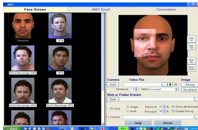
Partial face recognition. The square eye section is the partial. Numbers 3, 5, 6, 7 and 8 above are matches
